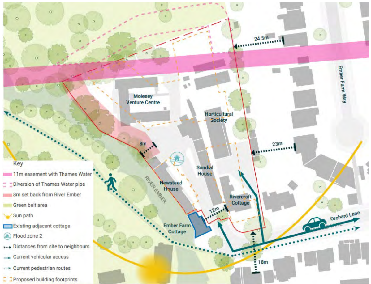
Figure 2.2 – Existing site layout
