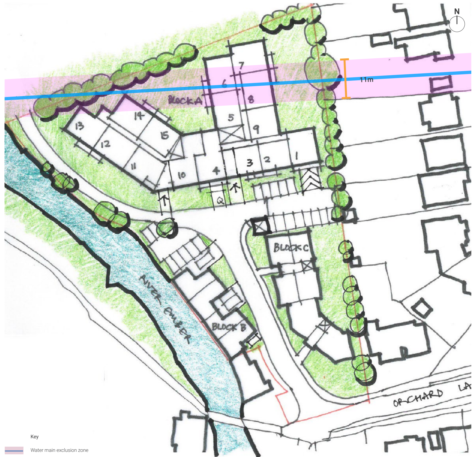
Previous ground floor plan shown at pre-app 3 with the water main and easement area overlaid
