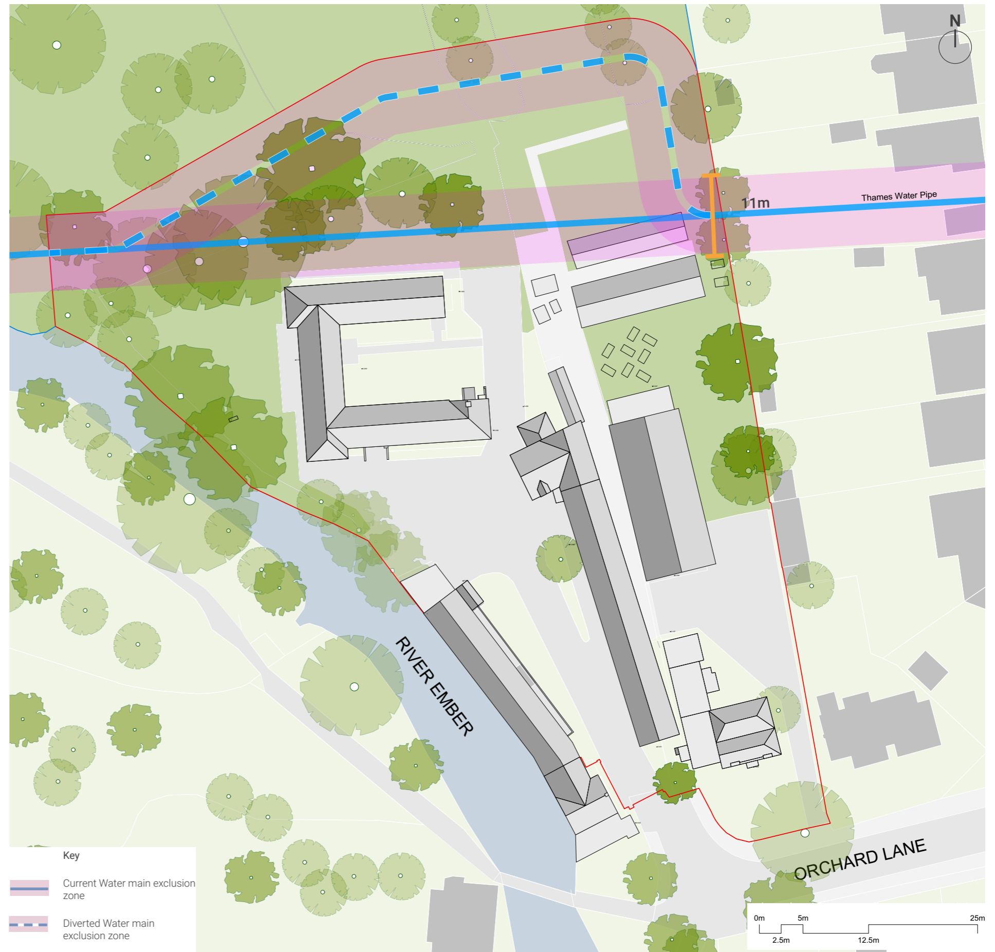
Existing site plan with current and proposed water main and easement area overlaid
