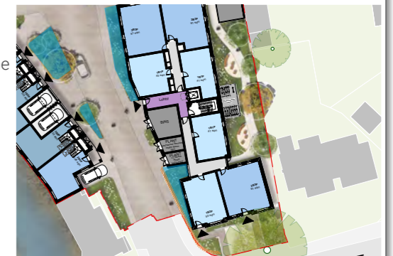
Ground floor of Building C showing defensible space
