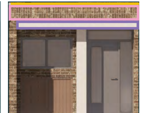
Building B entrance with stone lintel
