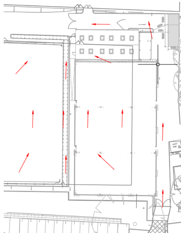
Figure 2 Existing Drainage Flow Paths
