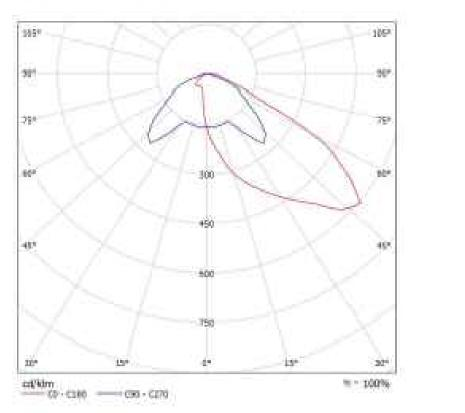
Due to missing symmetry properties, no UGR table can be displayed for this luminaire.
