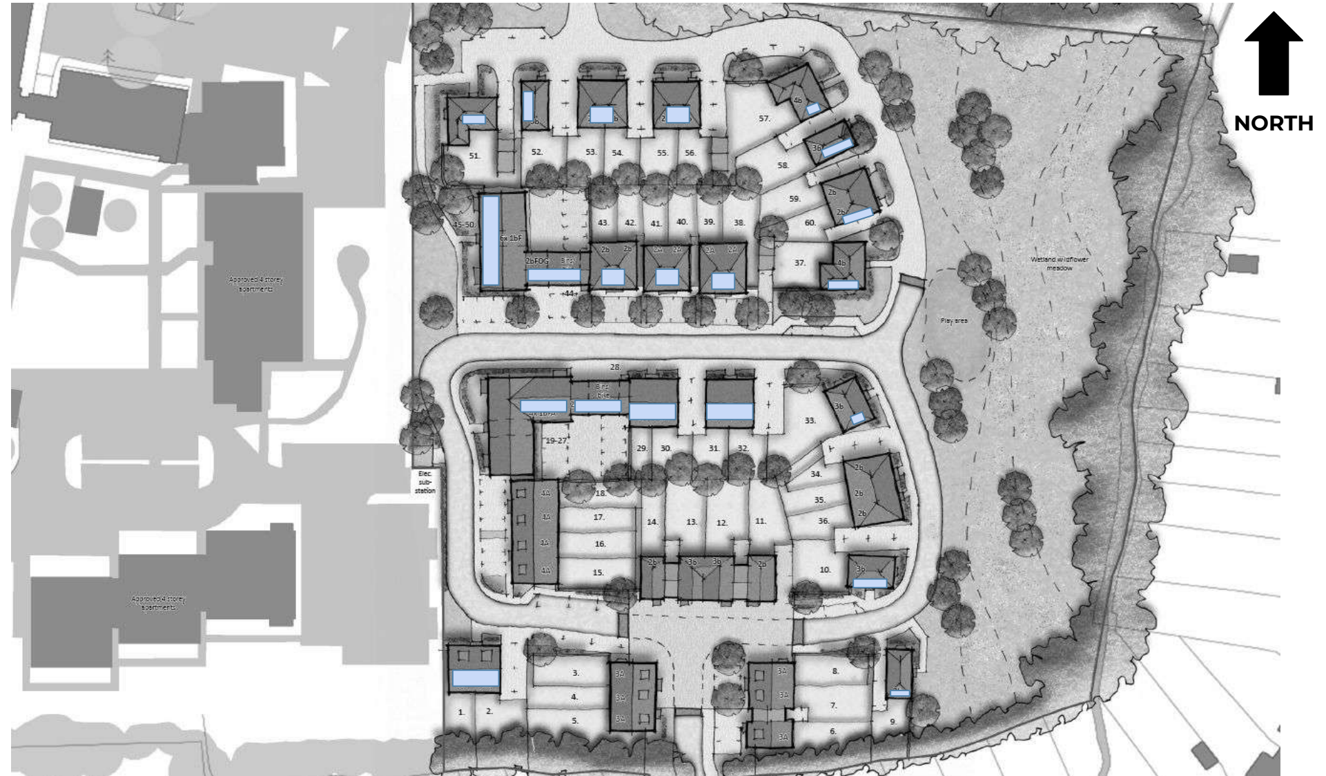
Figure 5: Indicative space for photovoltaic solar panel array location on the roofs of the proposed development (blue)
