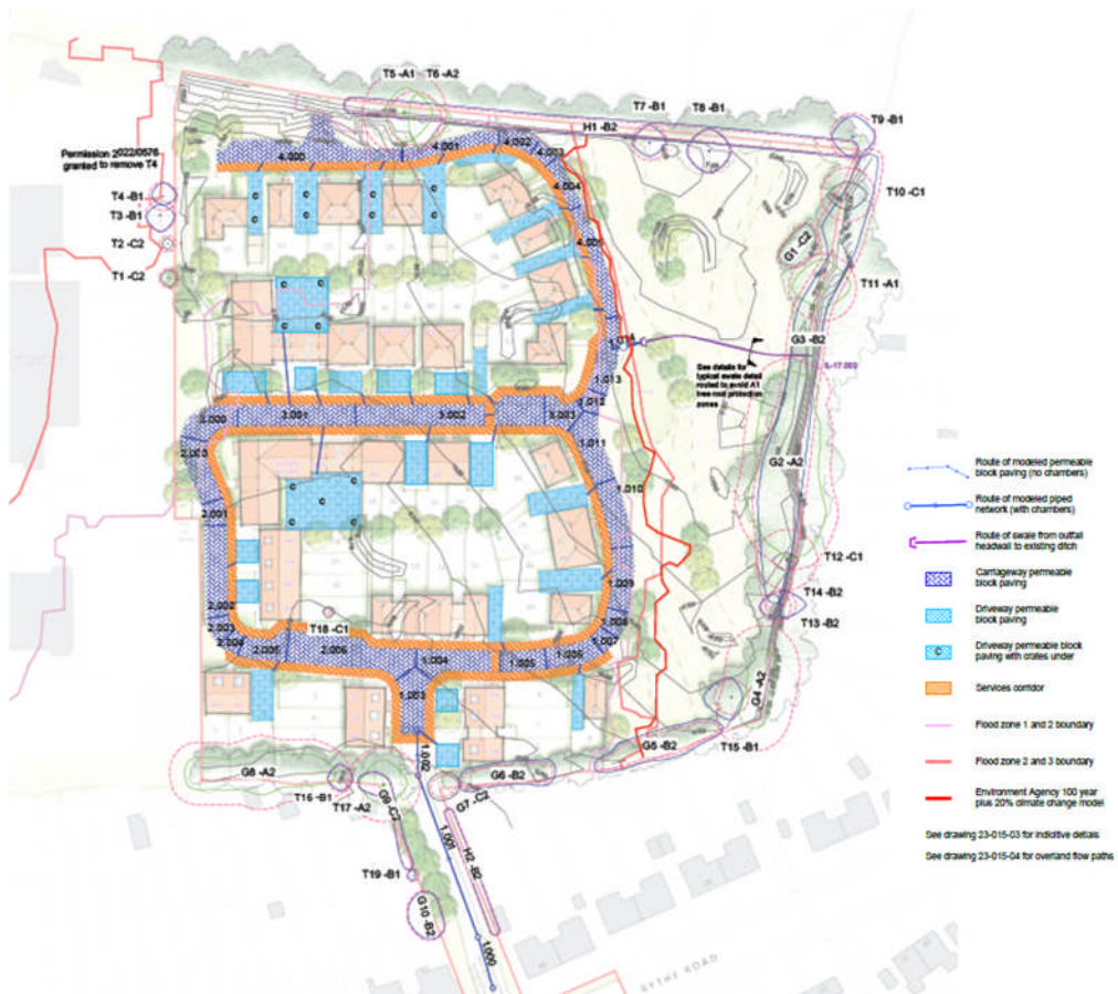
Extract of illustrative masterplan alongside flood risk information (source Appendix H of FRA)
