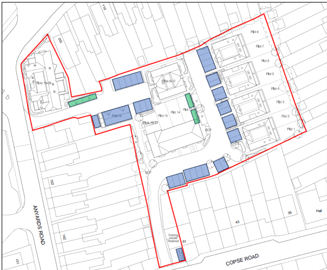
Figure 4.1 – Car Parking Locations (Spaces shown in blue with visitor bays in green)
